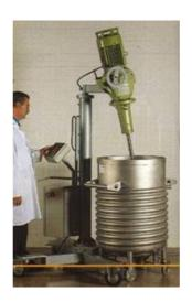
The direct drive technology forms the most important feature of the 10/20 series. A variable speed gear ensures there is the desired reduction factor with electric or pneumatic drives. This model is also equipped with remote control. If required.
