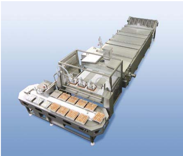
High performance egg peeling machine for 32.000 eggs/h
