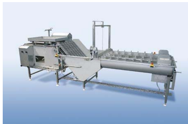
High performance egg peeling machine for 32.000 eggs/h
