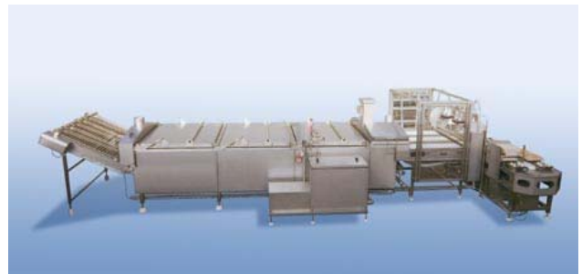
High performance egg peeling machine for 32.000 eggs/h
